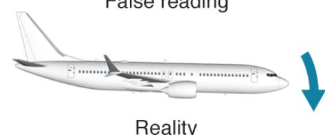
5. Pilots can temporarily switch off MCAS and pull up.
