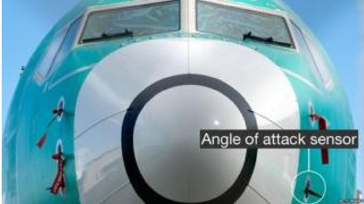
If this sensor gives a false reading, MCAS may activate and push the nose down when nothing is wrong.
